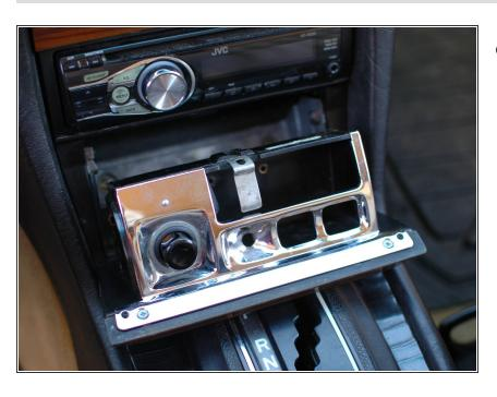
While continuing to hold down the tab you can pull the ash tray forward, and out of the opening it sits in.
