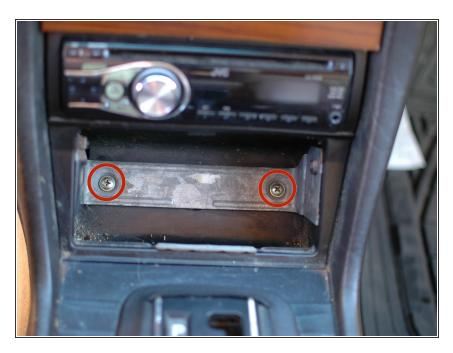
If you want to remove the entire assembly including the bracket that the ash tray rests in you can proceed to remove the two screws that hold it to the center console.
