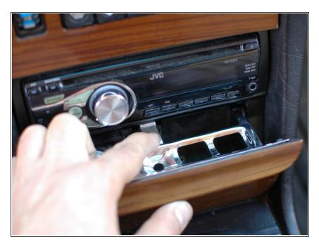
Now push down on the tab that is at the center of the ash tray assembly.
