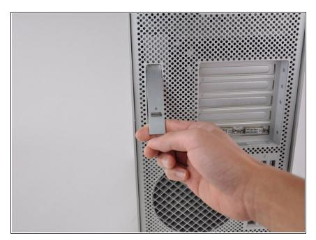
Lift the lever to unlock the case
