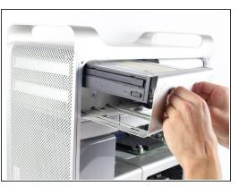
Firmly grasp the handles of the shown compartment and pull out firmly to remove the optical drive bay.
