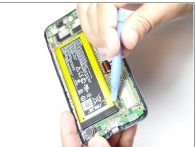
Using the blue plastic opening tool, gently disconnect the battery cable from the motherboard.
