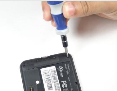
Remove the 13 - 3.6 mm screws using the Torx T5 bit in the screwdriver.
