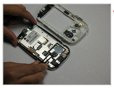
Pull the camera off the system by using the tweezers. Perform this step with caution.
