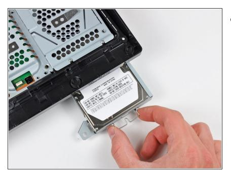
Using its attached metal handle, pull the hard drive out of its bay.
