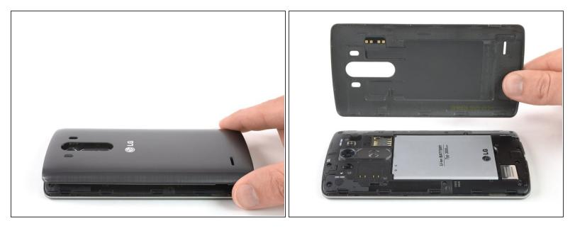
• Lift the back cover to release the rest of the plastic clips and remove it.
