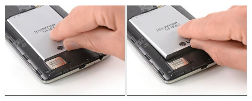
• Use a fingernail or a prying tool at the marked notch to lever the battery out of its recess.
