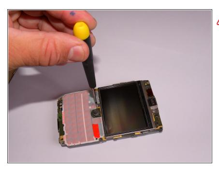
CAUTION! Remove the bottom screw with T5 Torx screw driver, not T6 !
