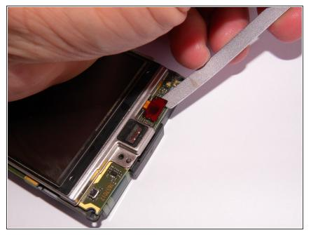
• Carefully disconnect the Flex cable connector. Then remove the display.
