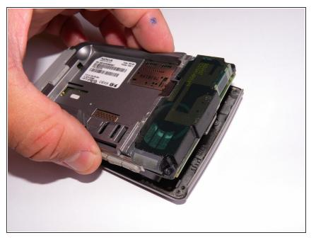
• Remove the assembly. The front cover will be released.
