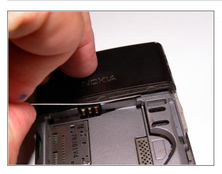
• Press the three latches to open this side of the cover.
