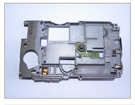
If necessary, you can replace the joystick, the button module or the connector housing.
