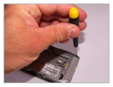
Remove the screws using Torx T6 screw driver.
