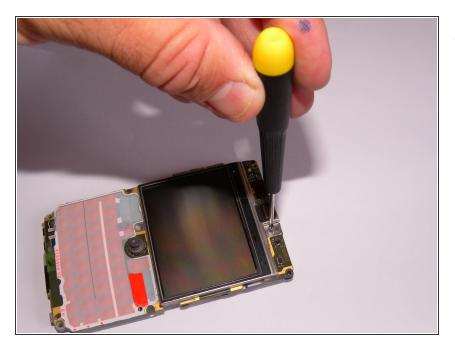
• To remove the display , unscrew the T6 Torx at top.
