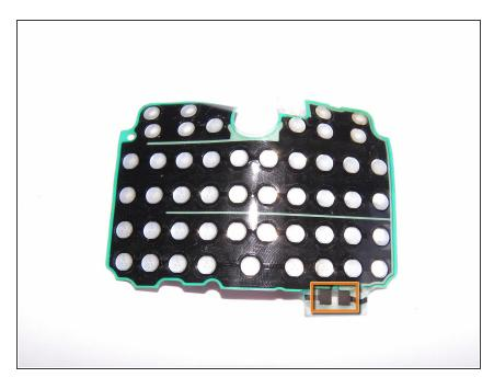
When you replace the keyboard membrane, align the two contacts at bottom.
