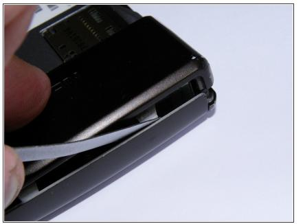
• To start, press one of the latches at the top of the phone to open the rear cover.
