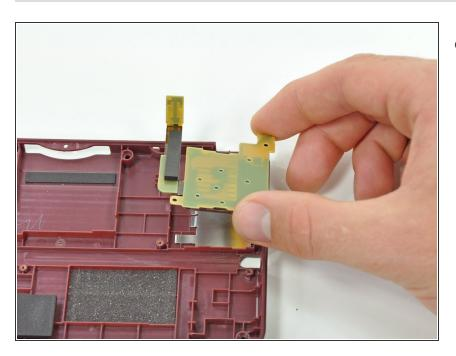
Lift the SD board off the lower case.
