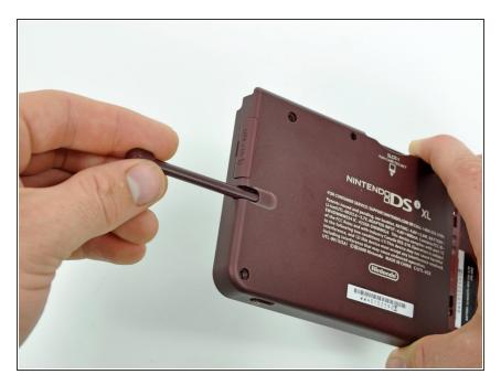
Remove the stylus from its housing on the right side of the DSi XL.
