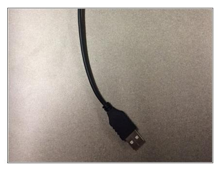
• Examine the cord for frays or any exposed wire that may cause a bad connection.
