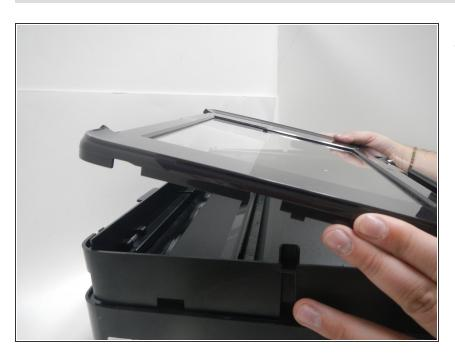
Lift the scanner glass piece from the printer.
