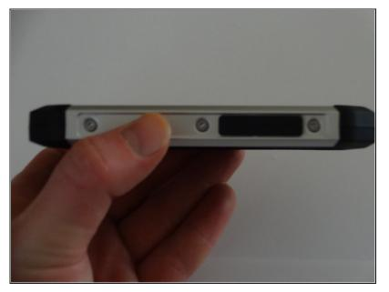
There are three remaining screws on each long side of the phone. A small hex bit is required for removal.
