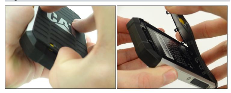
• Remove the back covering by gently lifting upwards from the bottom of the back covering. The back will snap off and the battery is exposed.
