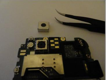
• Locate the camera module (pictured). To access the component to be replaced, the protective metal casing must first be removed. There are small gaps at each corner in which <u>tweezers</u> will fit. Choose any two, and slide this piece off.
