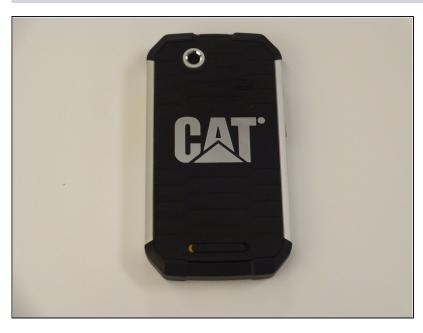
Place the phone screen-side down and place thumb on the yellow and black switch. Slide the switch to the right to unlock the back covering for removal.
