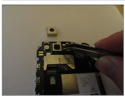
The module is also held in place by two small metal tabs to either side. To undo these, bend the bracket on both sides ever so slightly.
