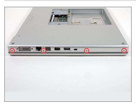
Remove the four 3.4 mm Phillips screws on the port side of the computer.
