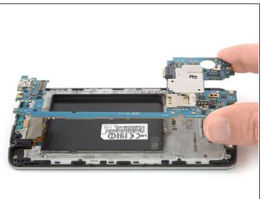
Grab the top section of the motherboard and carefully lift it out of the phone.
