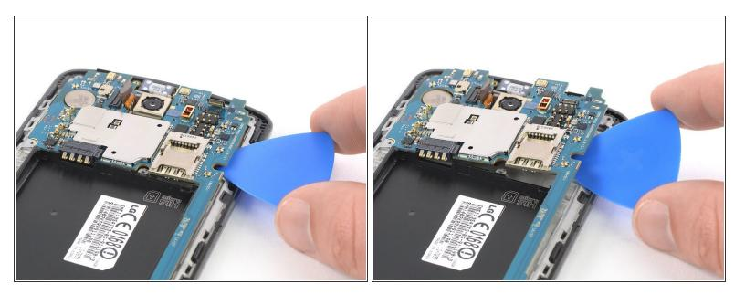
Slide the opening pick under the right edge of the motherboard where the SIM card slot is located and pry it up by rotating the opening pick sideways.
