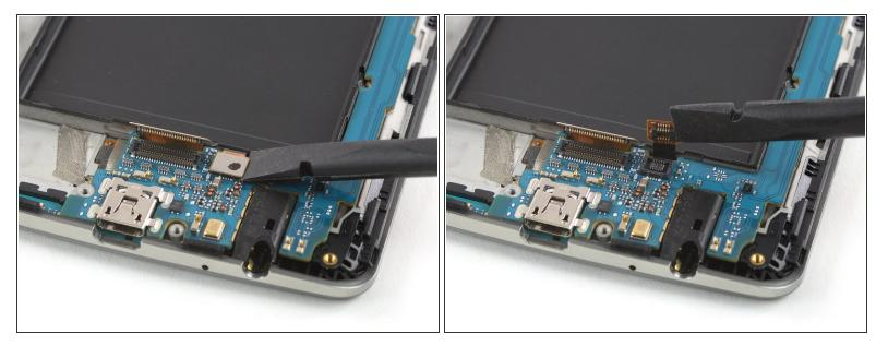
Use a spudger to pry up and disconnect the digitizer flex cable.
