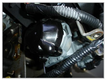
• Gently rotate the black cover aside and pull out the ignition switch.
