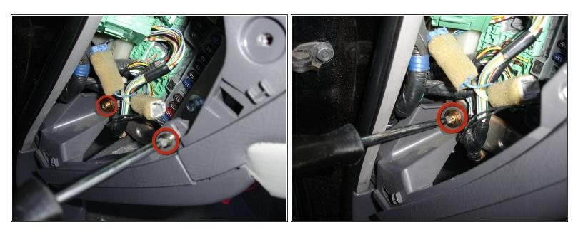
• Remove the two Phillips retaining screws that hold the driver's side lower panel to the dash.
