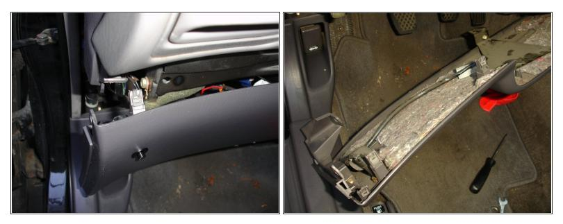
Now the driver's side lower panel can be removed. Begin on the left side and gently pull it off, so that all of the retaining clips are released.
