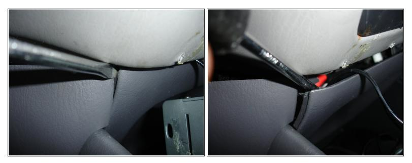
Use a flathead screwdriver to pry off the left side of the panel immediately below the radio surround.
