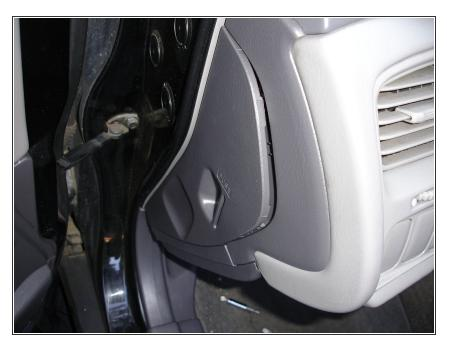
• Remove the driver's side fuse panel cover.
