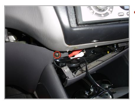
Remove the last Phillips screw securing the right side of the driver's side lower panel.
