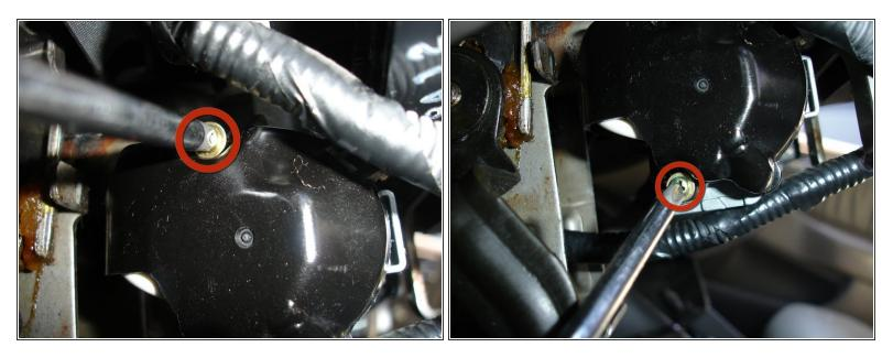
• Unscrew the two Phillips screws that hold the ignition switch cover (and switch itself) in place.
