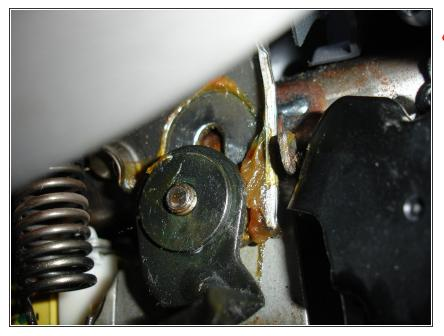
While in the general ignition switch area, make sure not to touch the steering column adjustment grease.
