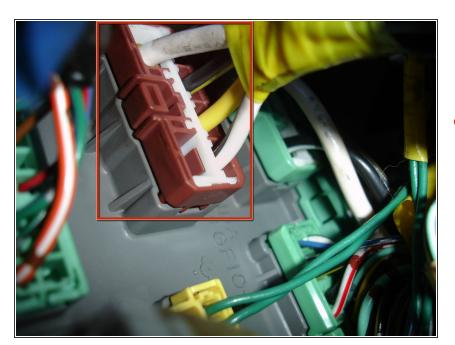
The ignition switch can now be unplugged for testing. The switch connects to the rear of the driver's side fuse panel. Shine a flashlight and find the connector highlighted in red.
