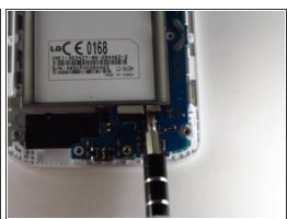
Use the plastic spudger tool or a flat head screwdriver to pry the ribbon cables off of their connectors.
