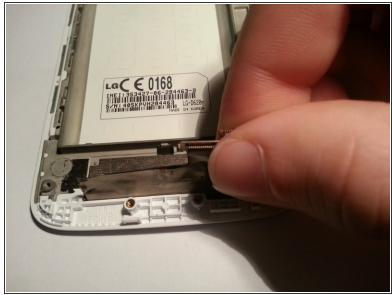
Peel the LCD cable off of the phone.
