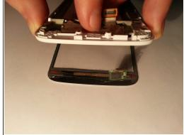
Push the ribbon cable connected to the Digitizer through the hole in the case and then pull the glass screen away from the phone.
