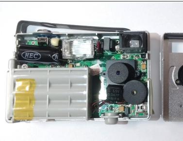
• Using a prying tool or fingernail, gently separate the back plate from the front plate, exposing the inside of the camera.
