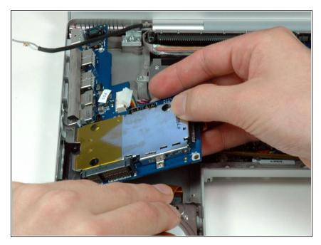
• Move the orange hard drive ribbon out of the way with one hand. Use your other hand to lift up the right side of the left I/O board and slide it out of the computer.
