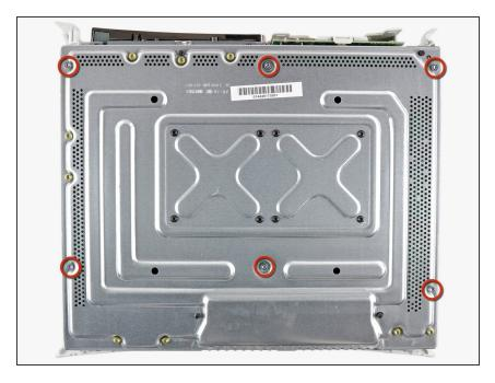
Remove the six silver 64 mm T10 Torx screws securing the upper case to the metal casing.
