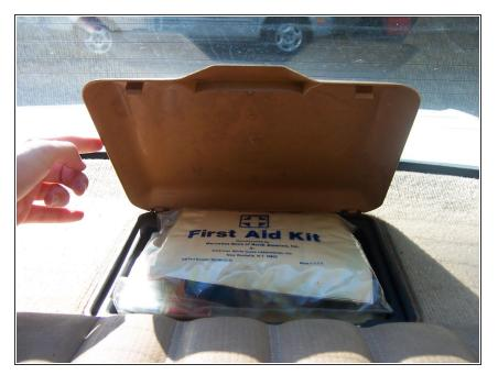
Before being able to proceed you will need to remove the first aid box. This guide does not cover this step, but basically, when you remove the first aid kit you will see several Phillips screws in the bottom of the box. Remove those and the first aid box lifts out.
