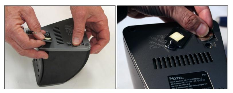
• Lift battery with fingers or using spudger
