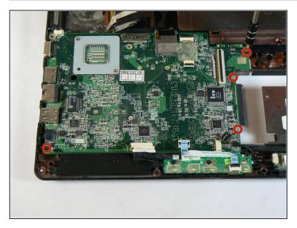
Unscrew the four remaining screws that are holding the motherboard in place using a PH1 bit. The silver screws are 5.6mm long and the black screws are 3.6mm long.
