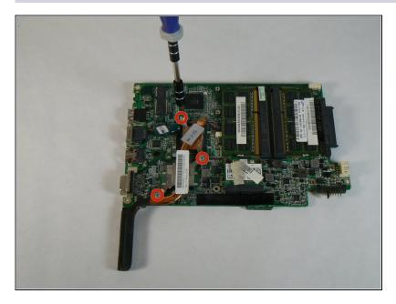
• Unscrew the three heatsink screws using a PH1 bit. These screws are attached to heatsink assembly.
