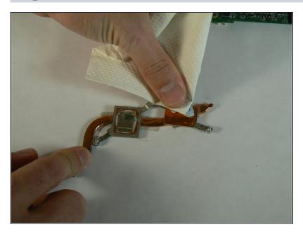
• Clean off the old thermal paste from the bottom of the heatsink. Using rubbing alcohol can make the process easier.
