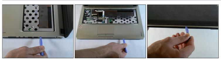
• Use the blue plastic opening tool to pry the silver plastic keyboard surround out from the black plastic bottom. You will need to do this around the entire perimeter of the laptop and will hear a pop every time one of the retention clips is unlatched.
