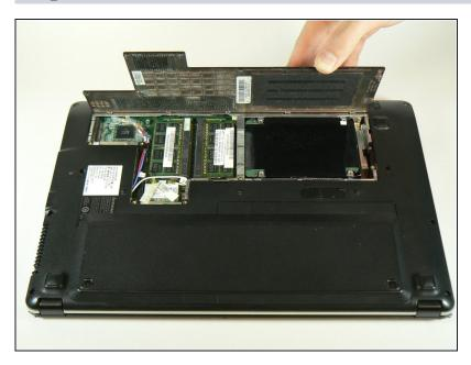
• Lift the back panel from the side closest to the battery and remove the panel.
