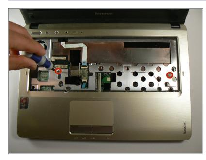
• Unscrew the two M2X3 screws that were under the keyboard.
