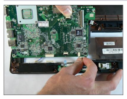
• Disconnect the remaining cable on the bottom right corner of the motherboard.
