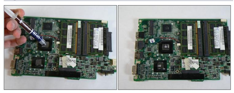
• Apply new, high-quality thermal paste to both dies. Noctua NT-H1 or Arctic Silver 5 are recommended. Only a small bead of thermal paste, roughly the size of a grain of rice, is necessary.
