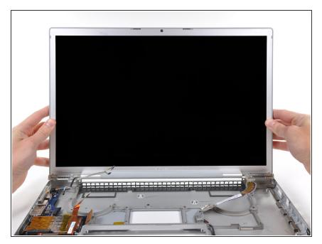
Grasp the display assembly on both sides and lift it up and out of the computer.
