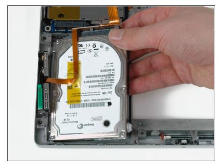
Lift the hard drive up from the right side and remove it from the computer. The Bluetooth assembly and orange ribbon cable are still attached to the hard drive and will come out with the hard drive.
