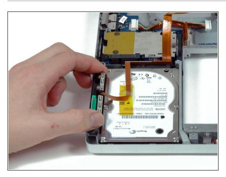
Lift the Bluetooth assembly out of its slot on the left side of the hard drive.
