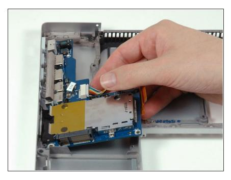
Lift up the right side of the left I/O board and slide it out of the computer.
