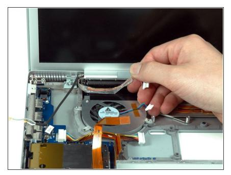
Peel up the iSight and inverter cables which are attached with a mild adhesive above the left fan.
