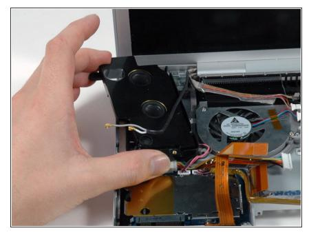
Lift up on the left speaker assembly and rotate it slightly. It is not possible to entirely remove the speaker yet, as it is still connected to the left I/O board beneath.
