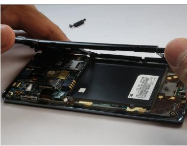
Pry the back panel from the frame of the phone to reveal the motherboard.
