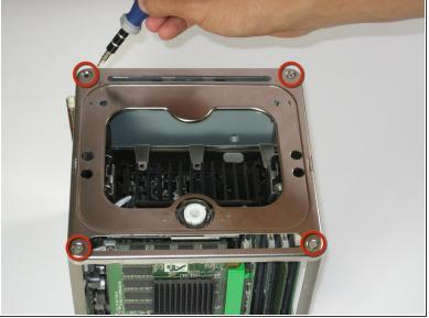
Place the cube upside down and remove the four T10 Torx screws on the front plate. Then remove
