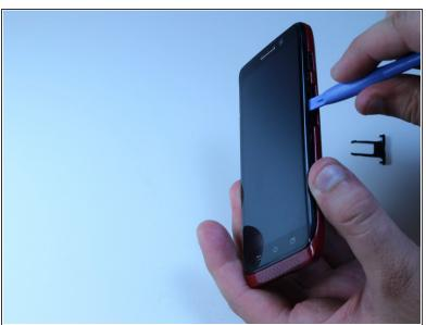
Pull out the volume keys using the iFixit opening tool.
