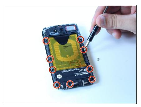
Use a T5 Torx screwdriver to unscrew the nine silver screws from the housing frame.
