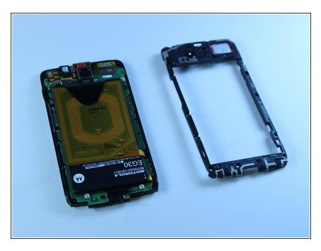
Carefully separate the housing frame from the motherboard.
