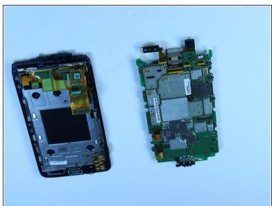
Carefully use the tweezers to separate the motherboard from the screen.
