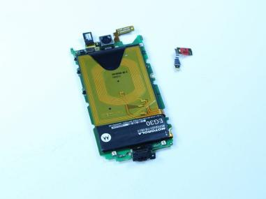
Carefully use the tweezers to remove the flash motherboard.
