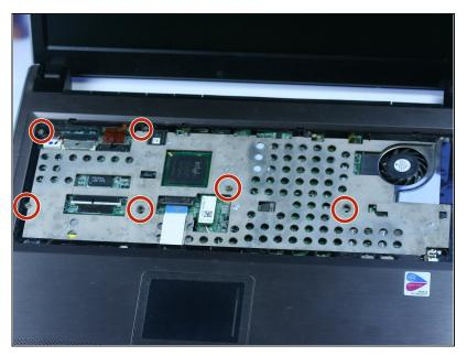
Remove the six screws from below the keyboard with a Phillips #0 screwdriver.
