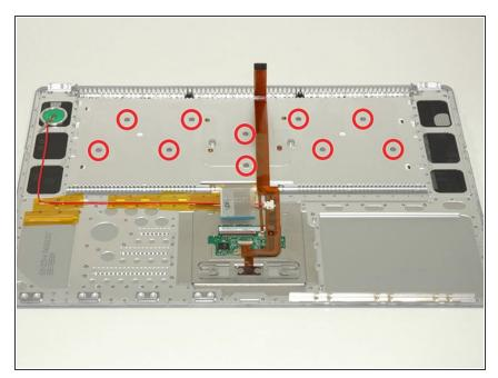
Remove the 10 identical Phillips screws attaching the keyboard to the casing.
