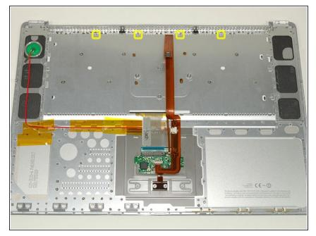
There are four locking tabs along the back edge of the keyboard holding it in place. These tabs must be straightened before you can remove the keyboard.
