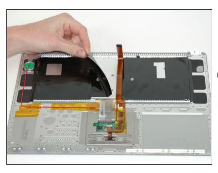
i On the following step, be careful with the tape on the side of the keyboard with the green power
