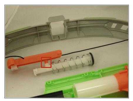
Make sure that plunger is reattached to the cocking mechanism.
