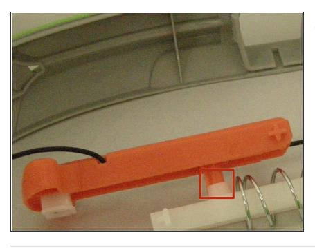
The cocking device needs to be attached to the plunger in order to function properly.
