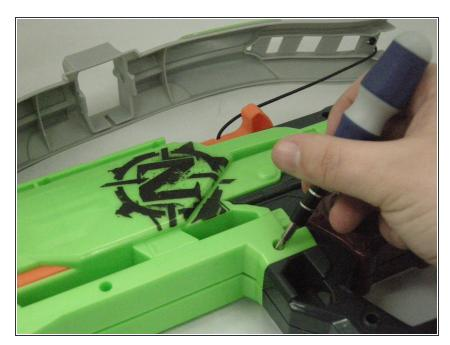
Use the screwdriver and unscrew each screw one-by-one placing each screw on the magnetic mat to insure they do not get lost.
