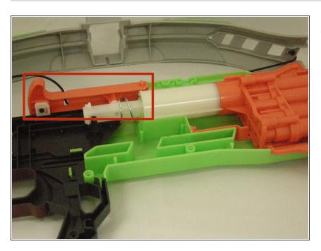
Make sure the cocking mechanism is properly aligned with the rest of the Nerf crossbow.
