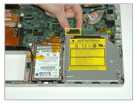
Disconnect the large black connector from the logic board.
