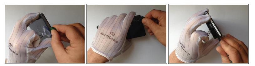
• Use a small suction cup and plastic tools for separating the Rear panel.
