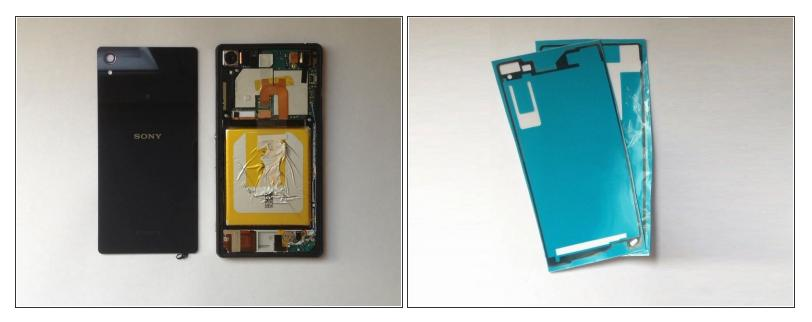
• Before installing the new cover, you must clean the phone from the old adhesive tape and install a new one (if your spare part has come without double sided adhesive tape).
