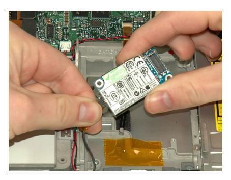
Lift the modem up and disconnect the remaining cable, at which point the modem will be free.
