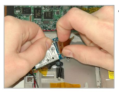
Disconnect the large orange ribbon cable from the top of the modem.
