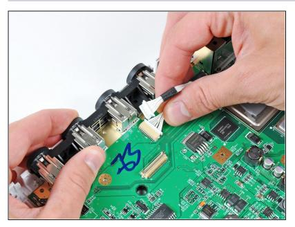
Carefully pull the DVD drive power cable away from its socket on the motherboard and remove it from the Wii.
