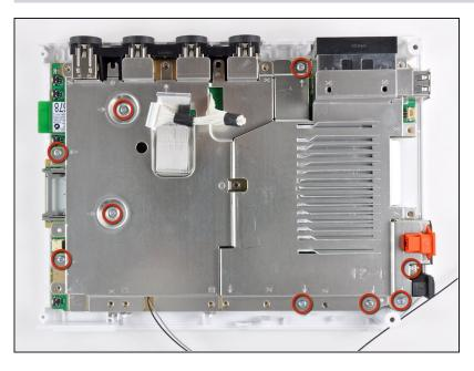
Remove the nine remaining 7 mm Phillips screws securing the motherboard cover to the bottom panel.
