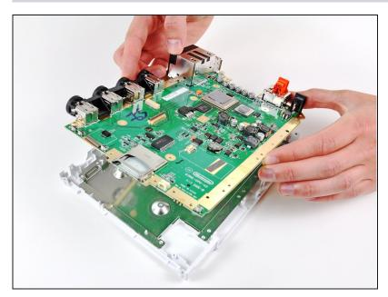
Carefully grab the motherboard by its edges and lift it off the bottom panel.
