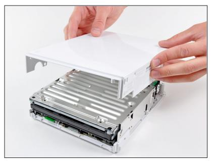
• Lift the outer case straight up off the body of the Wii.
