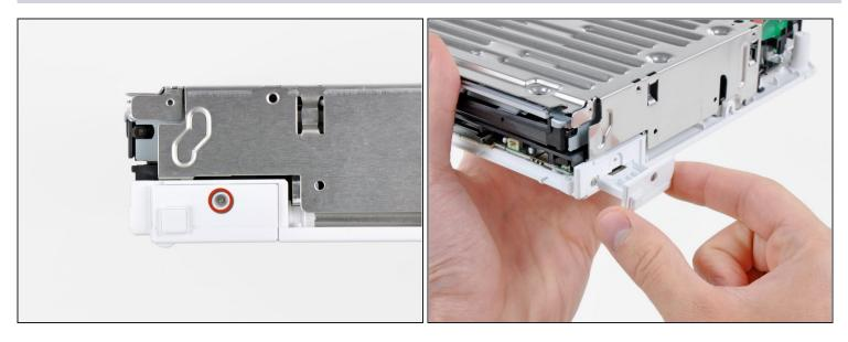
• Remove the small Phillips screw securing the battery door to the bottom panel.
