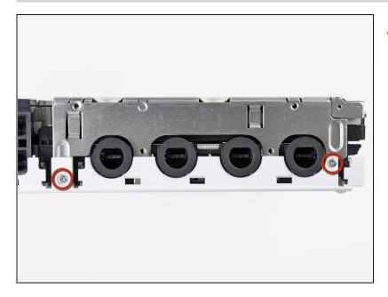
• Remove the two 8.2 mm Tri-Point screws securing the DVD drive shield near the controller ports.
