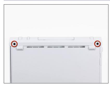
• Remove the two 8.3 mm Tri-Point screws hidden under the covers you just removed.
