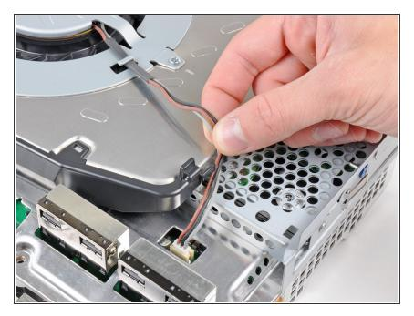
De-route the fan cables from under the plastic finger molded into the heat sink.
