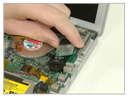
Lift the right ambient light sensor board Straight up from the Logic Board.
