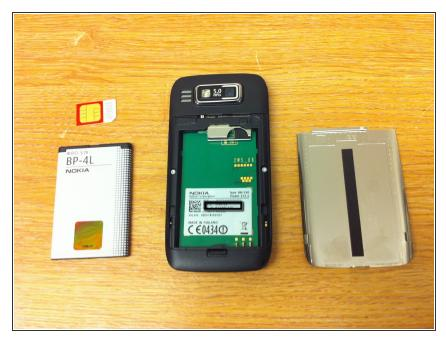
Remove metal backplate followed by the battery and then the SIM by pulling the SIM tray downwards. I do like this tray idea, but then again it's another thing that can go wrong with the device..
