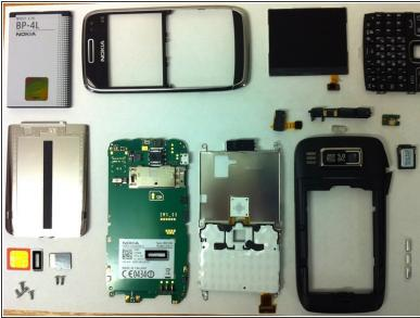
Ta-Da! This has to be the easiest phone to dissemble i have ever worked on. Only 6 screws on the entire device. Very good device i think personally, with this disassembly you should be able to replace any part in the phone without an issue.
