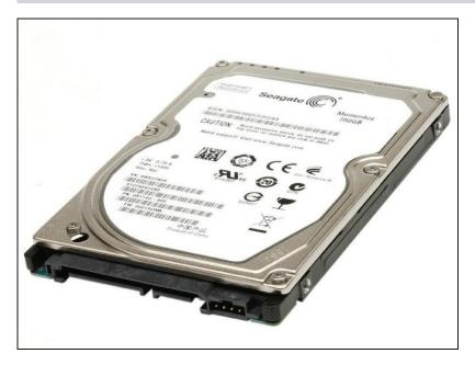
• Remove the 4 screws at the side and remove the HDD/SSD
