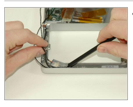
Using a spudger, pry up the Bluetooth board from the cavity in front of the battery compartment.
