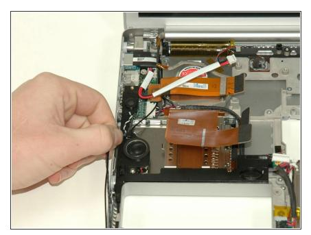
Deroute the Bluetooth and RJ-11 cables from around the left side of the speaker.
