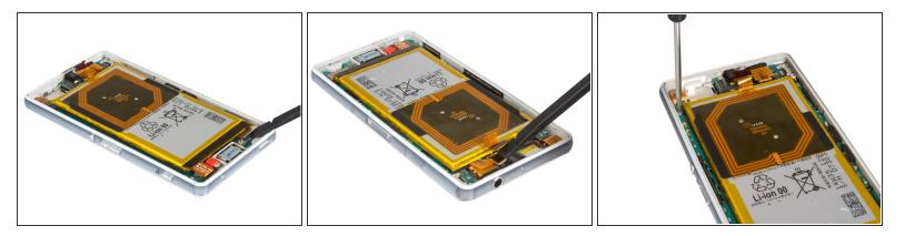
• Release all the connectors connecting with motherboard including the LCD screen connector and headphone jack connector. Undo the only screw on the motherboard.
