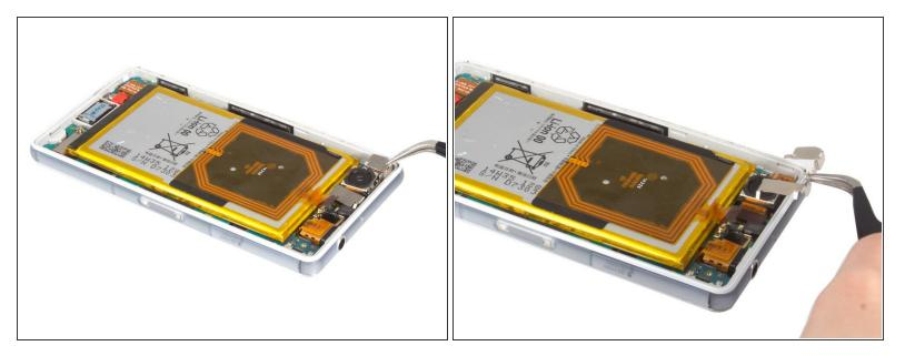
• Remove rear camera securing bracket.
