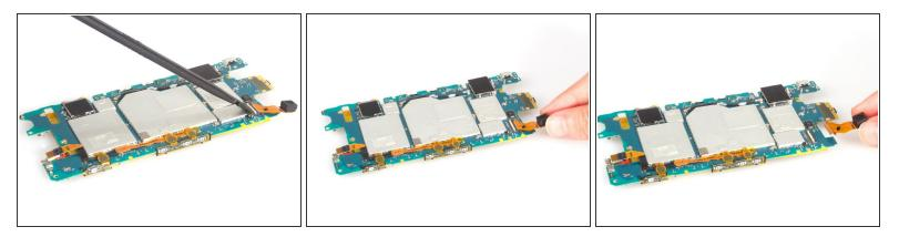
• Release the connector and remove the camera easily.
