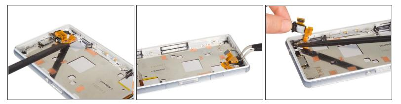
• Cut the adhesive under the flex and between headphone jack and midframe. And then pry up the sensors gently and remove the assembly finally.
