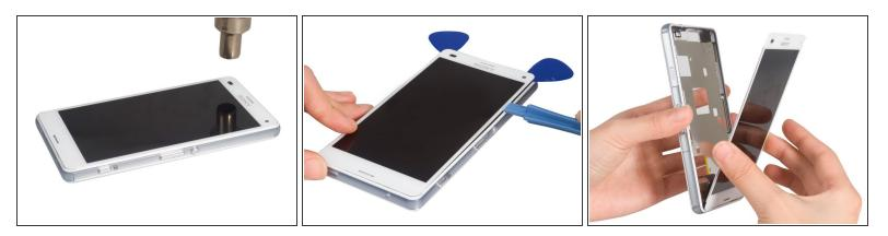
• Heat, cut the sticker and remove it. Notice where the earpiece is and be careful not to separate them when using the guitar pick. It's easy to break the earpiece.
