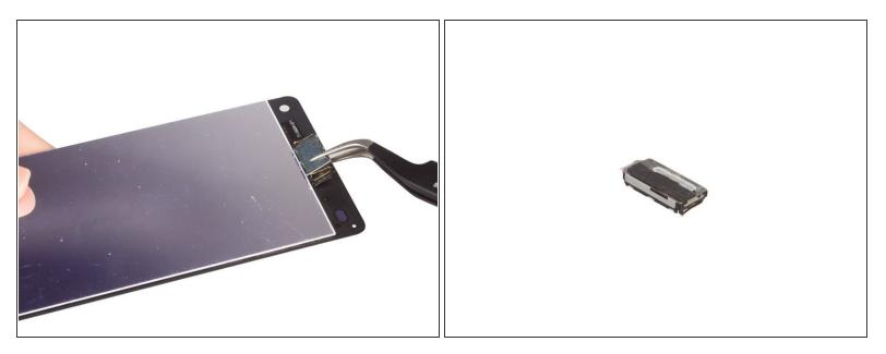
The earpiece is affixed to the touch panel directly, which is why it not recommended to separate it when disassembling the screen.
