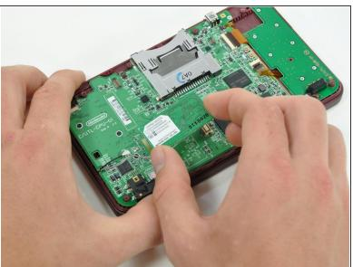
Lift the Wi-Fi board up off its socket on the motherboard.
