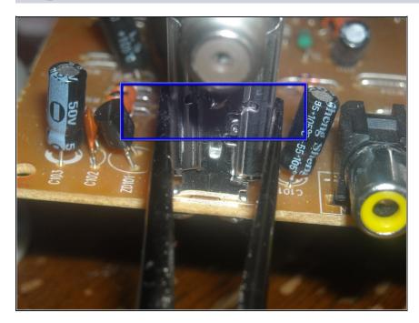
Re-seat both covers using needle nose pliers to ensure they're seated properly.
