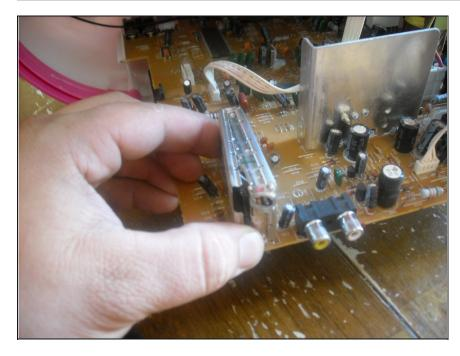
remove both covers on video input box, use a small prying tool if necessary, but you should be able to remove them by hand as seen here.
