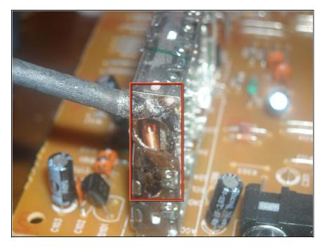
Use a soldering iron, and solder sucker to remove excess solder from the connector area. You can also use solderabsorbing braided wick.
