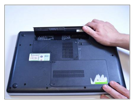
Carefully remove the battery from its compartment.
