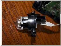
Light Globe Cover and the LED Module can be separated.
