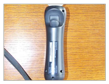
Remove the 4 screws holding the back over and trigger button on.
