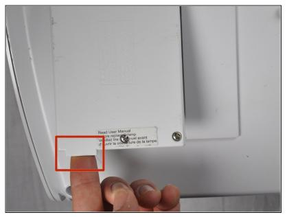
• Lift the panel off of the device.
