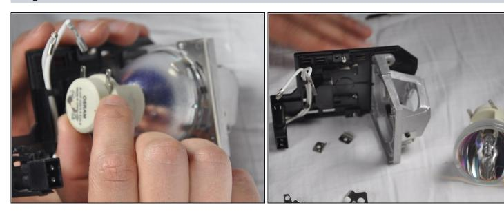
Remove the casing, then gently pull out the old light bulb and replace it with the new one.
