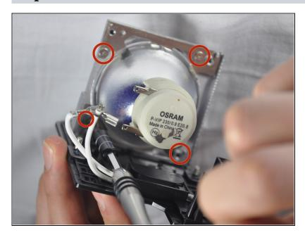
Remove the 4 screws on the back of the light bulb casing using a Phillips #1 screwdriver.
