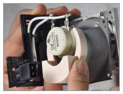
Carefully remove the light bulb insulator from the light bulb casing.
