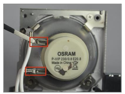
• Gently pull the wires off of the pins using tweezers.
