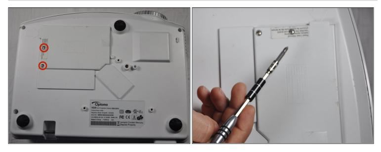
• Use a Phillips #1 screwdriver to loosen the screws that secure the panel on the bottom of the Optoma HD20.
