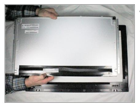
Lift up the screen to remove it from the plastic frame.
