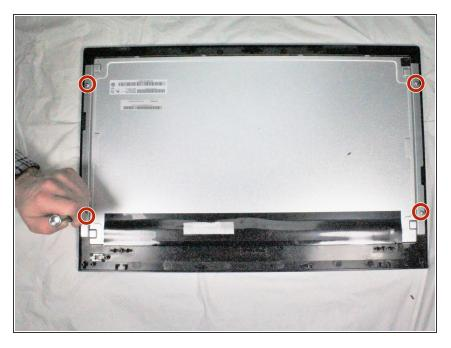
Remove the four, 12mm Phillips #2 screws from the outer edge of the back of the screen panel.
