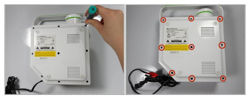
Flip the projector onto its back and unscrew the nine 15mm screws using the Phillips #0 screw driver.
