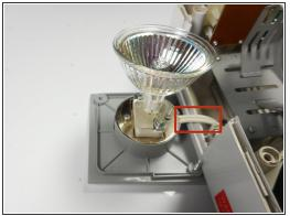
Remove the light bulb from its housing unit.
