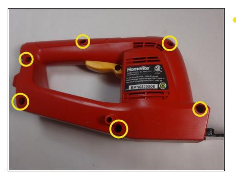
Remove the six 1.5 cm screws marked on the picture from the plastic casing with a Phillips #2 screwdriver.
