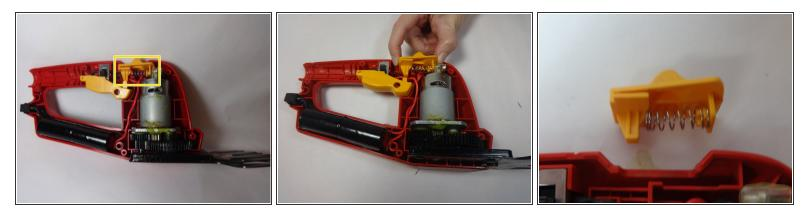
Remove the safety switch by pulling it away from the body of device.
