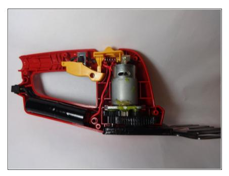
• Remove the faceplate to expose the inner mechanisms.
