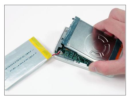
Lift up the end of the hard drive near the Firewire port to allow easy access to the battery connector.
